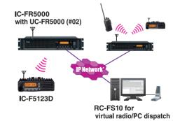
When using the IC-F5123D series in IDAS multi-site conventional mode, the IC-F5123D can communicate with other IDAS radio users working with other repeater sites and/or virtual radio/PC dispatch stations on the IDAS network.
